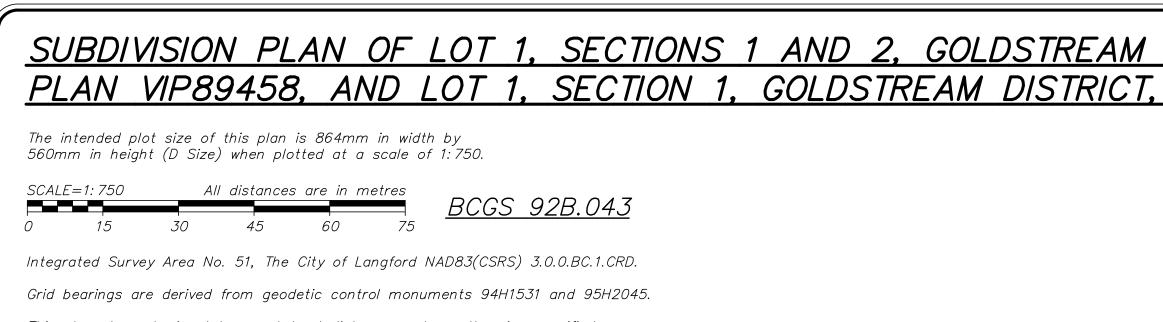
This plan shows horizontal ground-level distances unless otherwise specified. To compute grid distances, multiply ground—level distances by the average combined factor of 0.9996125 which has been derived from geodetic control monuments 94H1531 and 95H2045.
